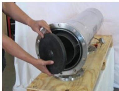
Figure 12: Removal of coarse screen cap
