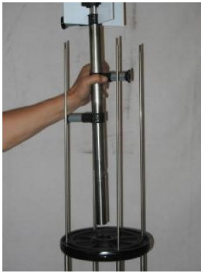
Figure 32: Removing the rotor assembly
