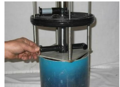
Figure 31: Removal of the hydraulic motor
