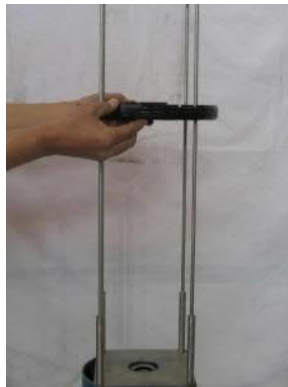
Figure 33: Lower bulkhead removal
