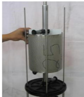
Figure 30: Removal of lower screen
