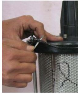
Figure 21: Removal of bulkhead seals
