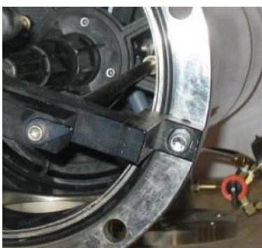
Figure 17: Puller shown bolted to the lid flange
