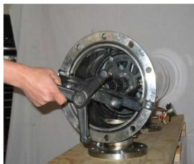
Figure 18: Removing internal assembly using the filter puller
