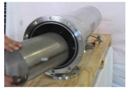
Figure 13: Removal of coarse screen
