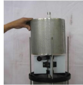
Figure 28: Upper screen removal
