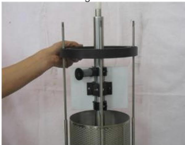
Figure 29: Removal center bulkhead
