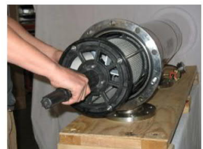
Figure 19: Removal of the internal assembly
