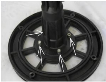
Figure 26: Reverser housing mounting screws
