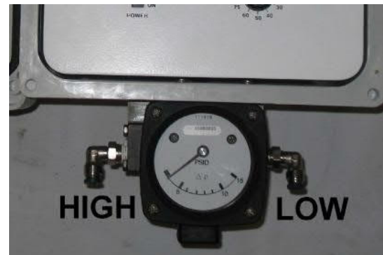
Figure 7: High- & low-pressure ports on the DP switch/gauge
