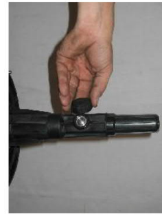
Figure 22: Removing pawl retainer.
