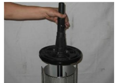
Figure 25: Removal of upper bulkhead
