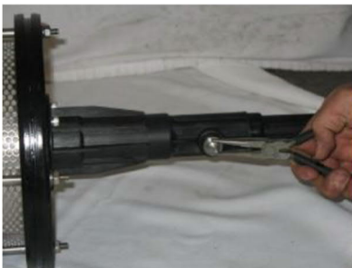
Figure 23: Removal of pawl
