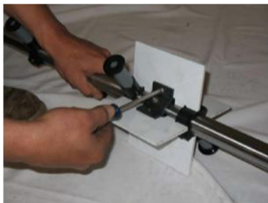
Figure 36: Removing the rotor paddles
