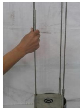
Figure 34: Removing lower sleeves
