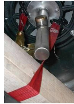
Figure 16: Alternative filter removal method
