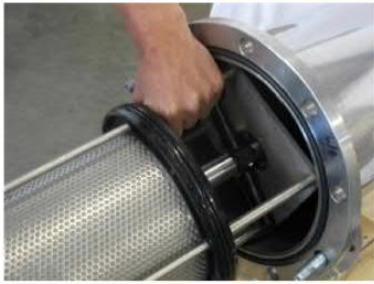
Figure 20: Supporting the internal assembly.
