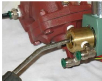
Figure 39: Blowing out the solenoid
