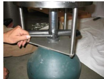
Figure 25: Removal of motor
