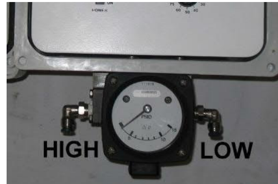
Figure 7: High- & low-pressure ports on the DP switch/gauge
