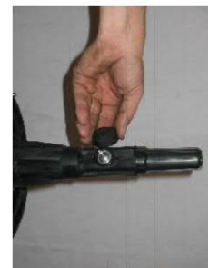
Figure 19: Removing pawl retainer
