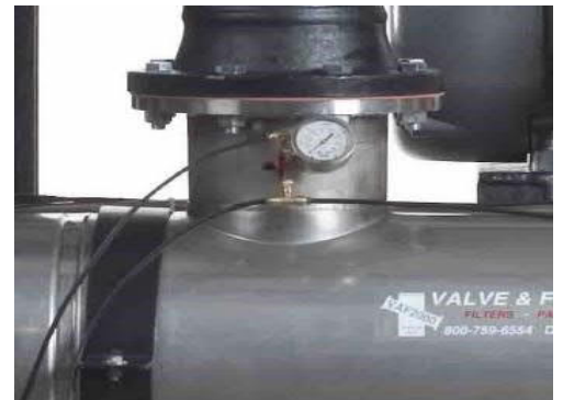
Figure 6: 3-Position manual valve and pressure gauge
