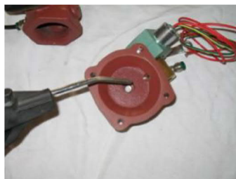
Figure 42: Removing water from cover plate
