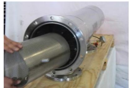
Figure 13: Removal of coarse screen
