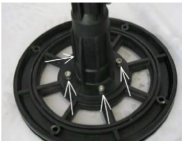
Figure 23: Reverser housing mounting screws
