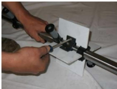
Figure 28: Removing the rotor paddles
