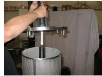
Figure 22: Upper bulkhead removal
