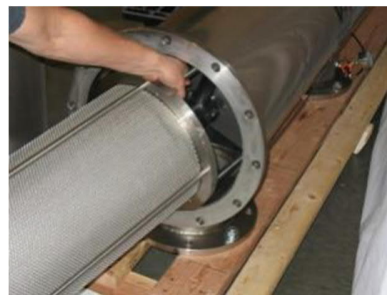
Figure 18: Supporting the internal assembly
