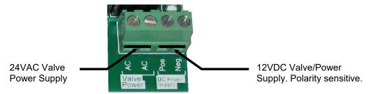
The EQ5 controller can be powered by 8 AA batteries (12VDC) or an AC Power module that supplies 12VDC to the DC valve/power input. When the controller is powered by only a DC power supply then only 9-30VDC latching valves must be used. If powered by the AC power module then 24VAC OR 12VDC or 9-30VDC latching valves can be used.
