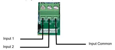
These inputs are Voltage free – do not apply voltage to the inputs.
